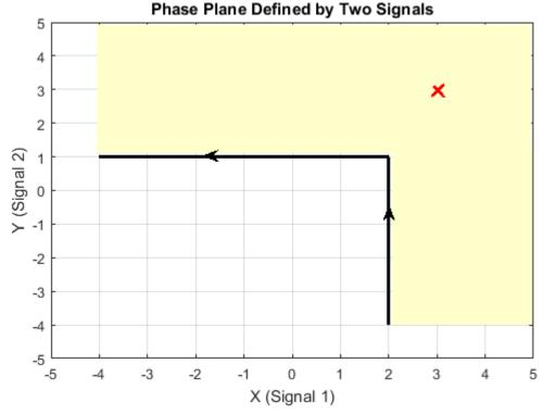
The plot shows that the edges were created in the opposite order. So, even though the requirement type is still '>=', the out-of-bound region, which is always to the right of the edges, is now flipped.
